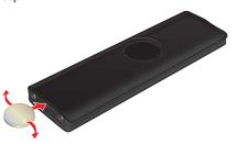
2. Insert the battery. The conductors of the battery must be in contact with the conductors in the housing.
