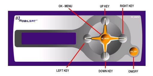
To activate operator menu press simultaneously the UP/DOWN keys for at least 3 seconds.
