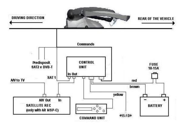
When the system has been connected correctly to a power supply, an auto test will be performed. If an error message appears on the display, look up the cause specified in the user manual.
